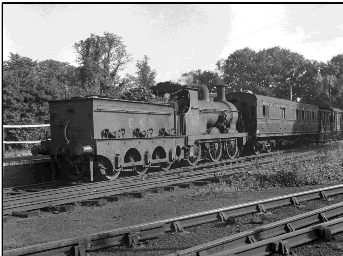
EKR 2, an ex SECR class O1 0-6-0, waiting with a mixed train at Shepherdswell, circa 1948. (LOS16251)
